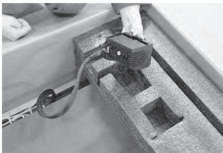
5. Take out the extruder and put it on the build plate. Be careful not to scratch the nozzle.
