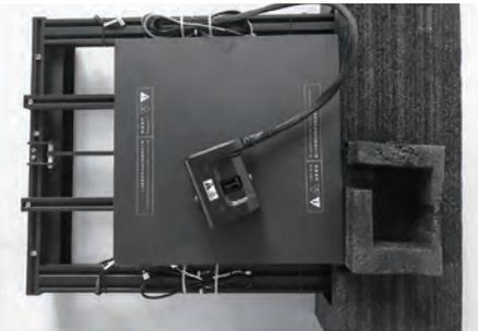
11. Remove the extruder and put it on the build plate. Be careful not to scratch the nozzle.
