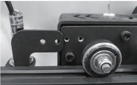
5. Put fixed seat on the right side of the extruder and fix it with 2 screws.
