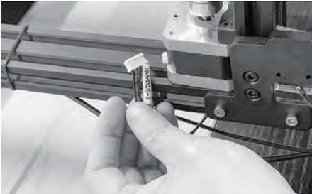
19. Find [Z-axis motor cable] on both sides marked with [Z-Stepper], insert them into Z-axis motor on both sides. Attention, the side of the plug with 2 protuberances should upwards.
