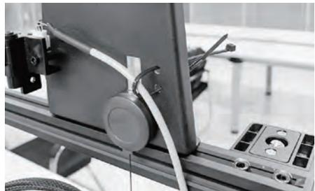
26. As is shown, fix [Filament detector sensor cable] with ribbons, hardware installation completed.
