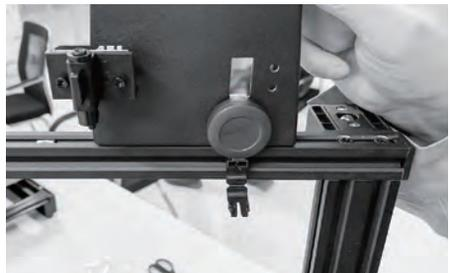
16. Take out filament fixed seat, and get ready for installing it on the top of the upper holder. Attention please, make sure the side of spool holder with the filament detector switch is facing the front of the printer.
