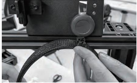
18. Clip extruder wiring harness into clips on the filament fixed seats.
