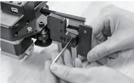
5. Slightly fasten the screw on the T-type fixed seat that has been unfastened before. But do not fasten with too much force.
