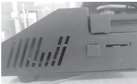
1. Insert memory card into equipment card slot.
