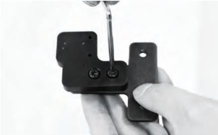
3. Slightly unfasten the screw on the T-type fixed seat, thus the T-type screws at the back of the fixed seat is movable.
