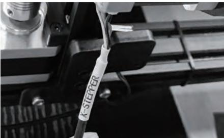
20. Find [X-axis motor cable] marked with [X-Stepper], insert it into X-axis motor. Attention: X-axis motor cable socket is under the motor, the side of the plug with 2 protuberances should upwards.
