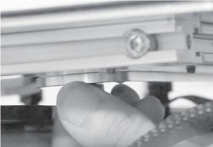
1. Tighten the four nuts of the build plate counterclockwise
