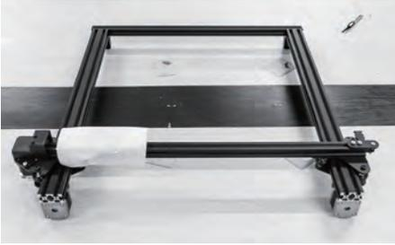
1. As is shown, take out the upper holder on the table and remove protective foam.
