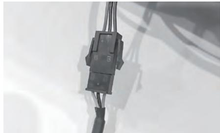
6. Connect sensor plug with sensor cable at the back of printer LCD.
