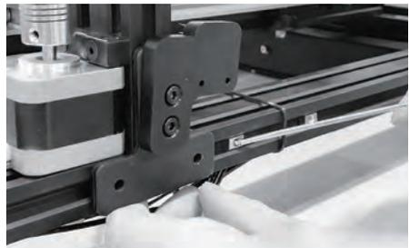
11. As is shown, adjust 4 T-type screws (two on each side) to screws holes of T-type fasteners for subsequent fixing of T-type fixed seats on both sides. (Find T-type screws in the sliding slot on both sides).
