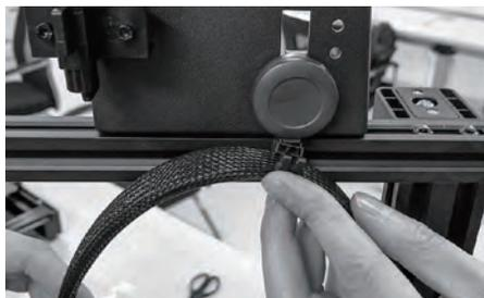
7. Clip sensor cable into pulley clip on the top of filament fixed seat for sensor cable is too long.
