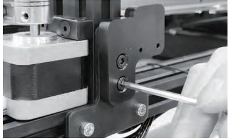
13. Tighten screws on the T-type fixed seats.
