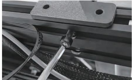
8. Insert upper holder into L-type block on both sides.
