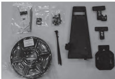
9. Check parts of the tool box: tool kit, memory card, screw bag, filament, ribbons, filament fixed seat, filament support, T-type fixed seat of Z-axis, T-type fixed seat of Z-axis+Sensor.
