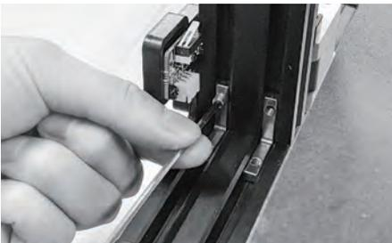
10. Use 8 M4\*5 set screws to fix L-type block, four on each side.
