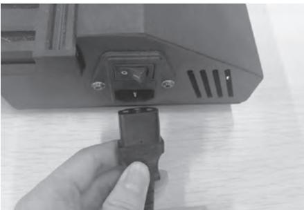
5. Insert power cable into supply socket on the left of the printer.
