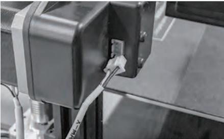
23. As is shown, find [X-axis sensor cable] marked with [X-Max], insert it into the X-axis sensor socket at the back of X-axis motor. Attention: The side of the plug with two protuberances should be oriented to the back of the printer.
